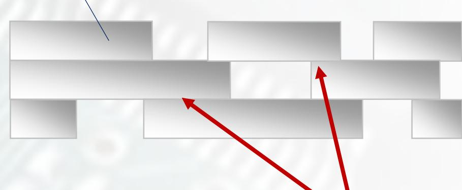
**Larger particles makes particles easy to contact**
